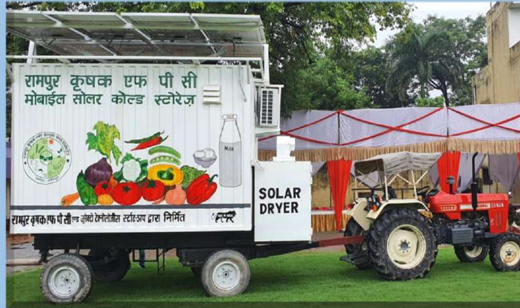
2 Solar Mobile Cold Storage Capacity: 20 MT each. Solar Dryer : 0.5MT MFD by FPC
